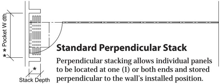
Perpendicular stacking allows individual panels to be located at one (1) or both ends and stored perpendicular to the wall's installed position.
