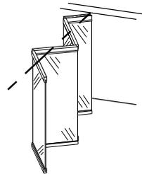
**Continuously Hinged Center Stack (Centerfold)**
