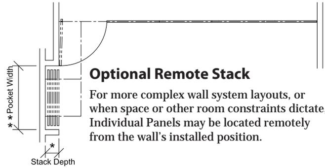
For more complex wall system layouts, or when space or other room constraints dictate, Individual Panels may be located remotely from the wall's installed position.
